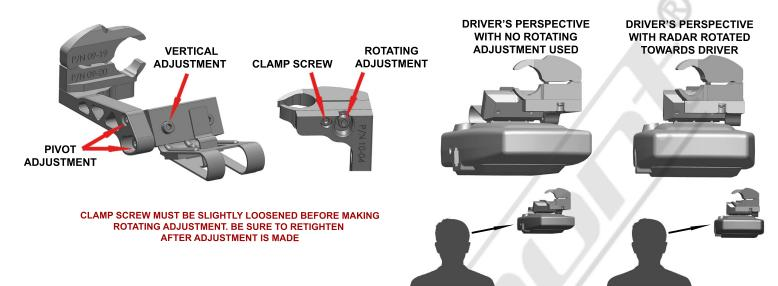
4 - Install your radar detector onto the mount. Use the adjustments shown above to adjust the RD to your desired position. We recommend adjusting the RD as close to the bottom of your mirror as you can. **NOTE** When the rotating adjustment is used to rotate the RD towards the driver, the footprint of the RD is reduced as shown above. Be sure to tighten all of the adjustment screws after the adjustments are made.
