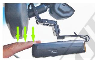
**5** - If the RD is too close to the bottom of the mirror, You may access the buttons on top of the RD by gently pushing downward on the front of the RD with one finger and push the desired button with another finger. Then allow the RD to return to it's original position by gently letting it spring upward. When accessing the buttons, be sure to push the RD downward just enough for your finger to fit between the RD and mirror. **Do not push down more than what is needed.**
